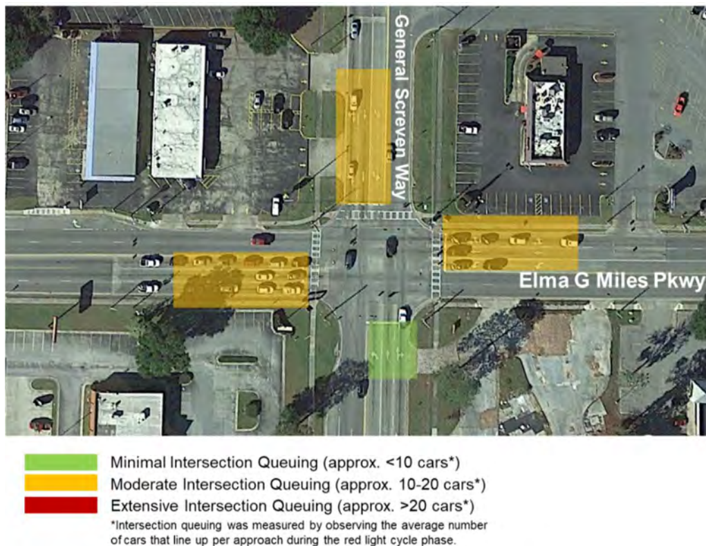
FIGURE 10: E.G. MILES PKWY AT GEN SCREVEN WAY EVENING PEAK PERIOD INTERSECTION QUEUING
