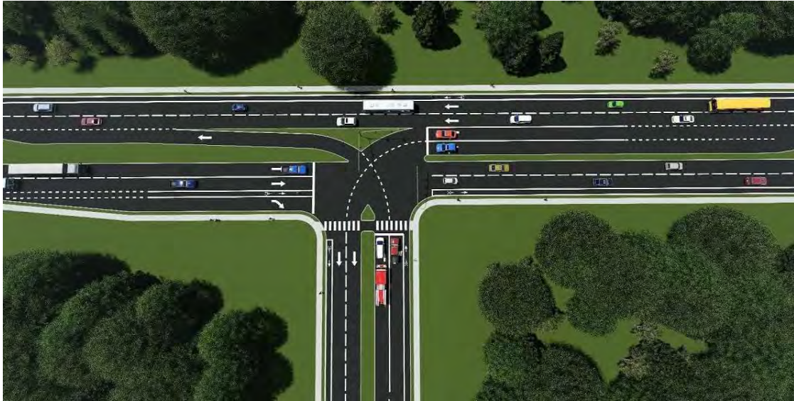
FIGURE 46: EXAMPLE OF A HIGH-T INTERSECTION
