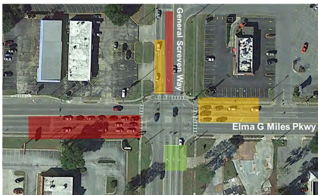
FIGURE 9: E.G. MILES PKWY AT GEN SCREVEN WAY MORNING PEAK PERIOD INTERSECTION QUEUING
