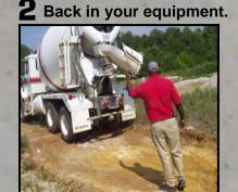
Washdown only the chute, hopper and rear of the vehicle. Do NOT wash out the drum.
